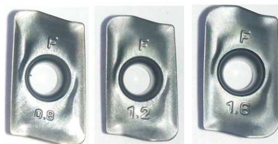
Figure 6.1: Inserts Used (Nose Radius: 0.8 Mm, 1.2 Mm And 1.6 Mm)
