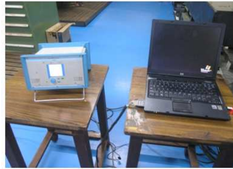
Figure 8.2: Amplifier and Computer Used for Force Measurement
